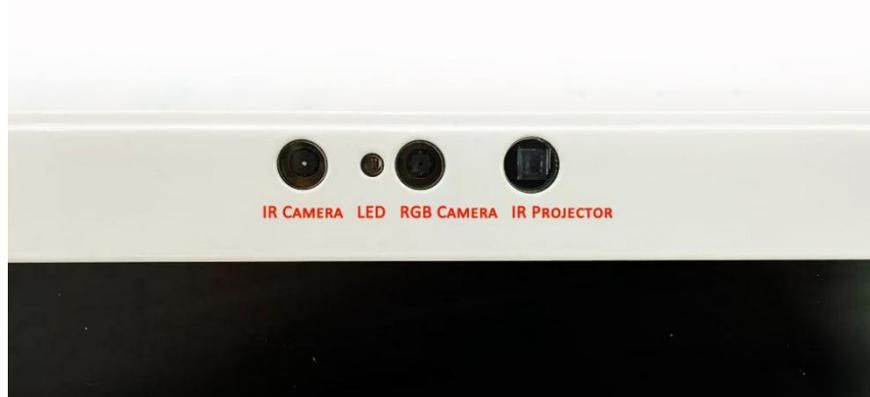
Best view distance is about 100 cm. The eye tracking sensors easily find the viewer and track his/her movements. The eye tracking and imaging algorithm are based on AI deep learning to manipulate the relative 3D maps in a fast and accurate way. The viewer in front wouldn't find any hint of the image adjustment, because he/she is always at the best 3D watching angle.
